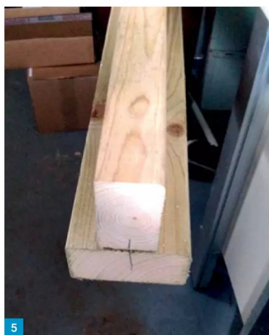
Fig. 1: Squeezing a base into the available space. Fig. 2: The rear was built horizontally ... Fig. 3: ... and then braced in its final position. Fig. 4: The completed cladding with gaps for door and window. Fig. 5: Composite beam for roof support.
