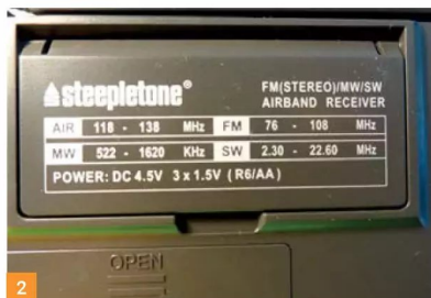
Fig. 1: The front of the (larger) Steepletone MBR1051. Fig. 2: The frequency coverage offered by the Steepletone MBR1051.
