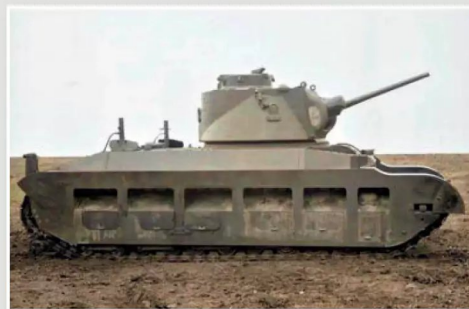
◀ A12E1 Matilda Mk I: This A12 prototype featured six mud chutes twin AEC 87bhp engines and a Vickers heavy MG
