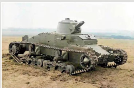
◀ A11E1 Matilda Mk I: This early prototype tank featured one Ford V8 70bhp petrol engine and a Vickers MG
